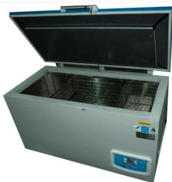
**Multi air-flow plenum system** ensures excellent temperature uniformity in larger capacity models.
