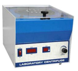
We are listed at the apex as a **Centrifuge Machine** Manufacturer and Exporter from India. Our rectangular Centrifuge Machine is high speed machine that comes with a digital meter and timer. The Centrifuge Machine (Electrical) Model GE- 160 has the bowl and cover made of heavy gauge spun Aluminium to completely enclose the head and enhance its functioning.
