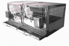
**Door:** Cage has two doors and each door has a fixed label holder and arrangement for fixing water bottle and food hopper. The door will be made of wire mesh of 2.5mm x 5mm SS rod welded on a frame of 5mm SS rod and covered with 22swg SS sheet.
